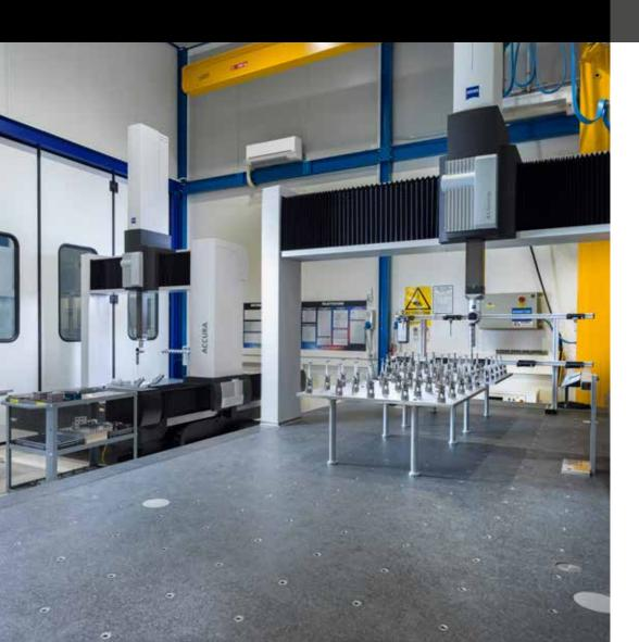
All inspections are performed at a room controlled temperature of 20°C / 68°F
